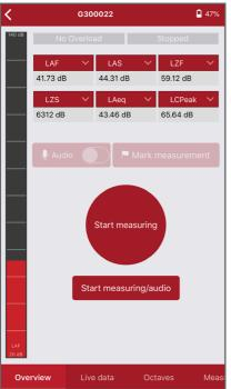
This screen is the default home screen for dBActive and displays live noise data for a number of parameters, each of which can be changed. Press the arrow on the value you wish to change. A menu will appear allowing you to select the value you wish to see (see image below).
