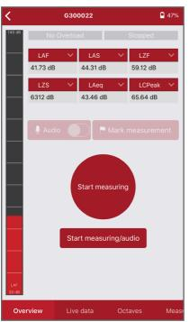
From the overview screen, choose either 'Start measuring' or 'Start measuring/audio' to begin a measurement. If you choose 'Start measuring/audio', the measurement will include an audio recording of the noise. If you choose 'Start measuring', audio will not be recorded.
